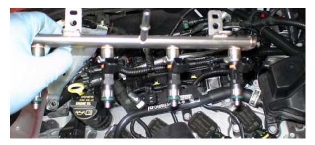
NOTE: Tilt the injector rail into a catch pan and drain excess fuel from the rail.
