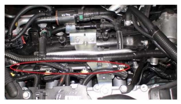
Description: Fuel rail is about 12 inches long, 1 inch wide, and 0.5 inch thick. Upon close examination, you will see 4 injectors attached to the fuel rail; and connected to each injector is an electrical plug. The fuel rail is held onto the intake manifold via 2 black screws with torx (6 point female) heads.
