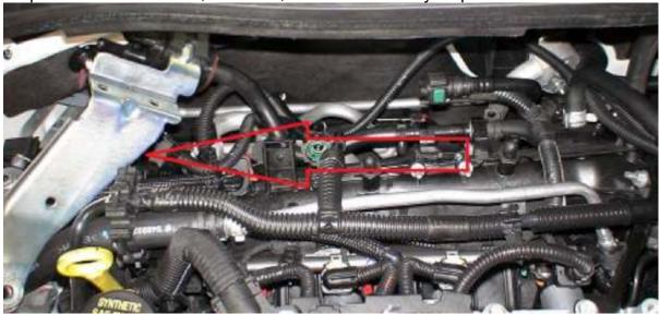
Step 2e: Return to the fuel feed hose and disconnect the hose from the fuel rail. Note, first slide BLUE retaining clip, then squeeze the grey / white tab to release the quick disconnect fitting. Finally side the hose out of the fuel rail as pictured. Slight amount of fuel will drip from the hose and rail.
