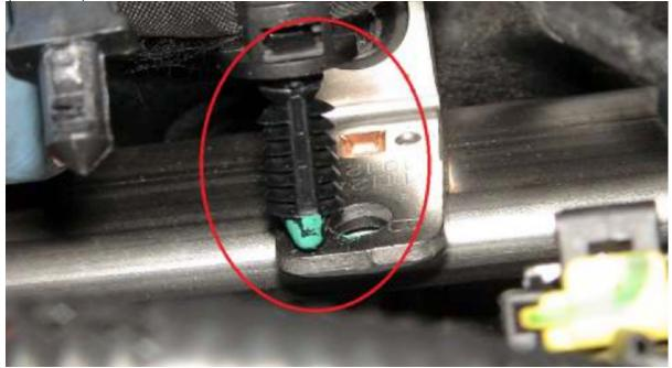
• Step 2h: Pull the injector loom up and out of the way.
