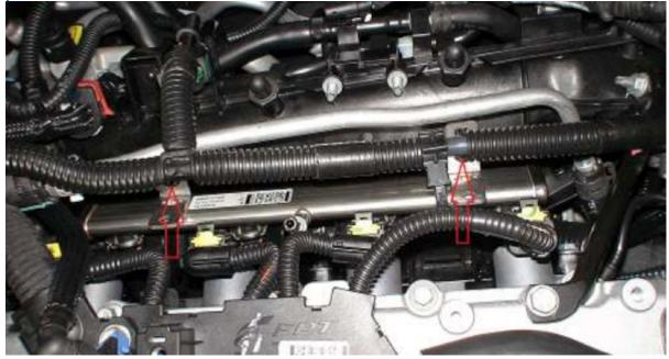
Remove the left screw with T27 Torx driver.
