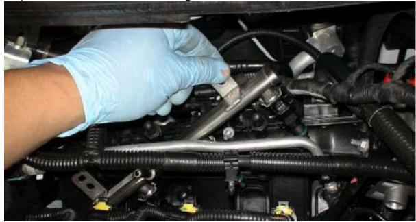
• <u>Step 4: Install the fuel rail onto the engine in reverse order.</u>
