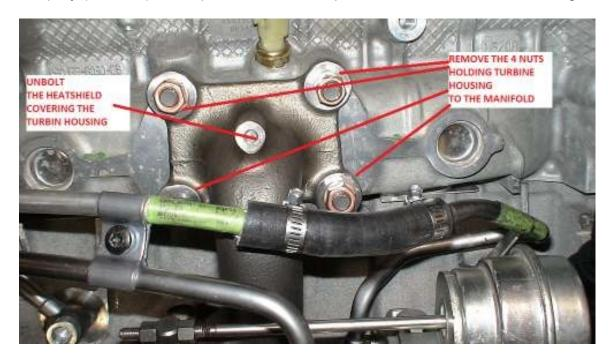
i. Remove the disconnected turbo assembly from the vehicle.
