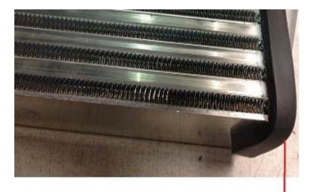
At each corner, ensure that the cushion tape wraps around to the top and bottom surfaces around the corners.
