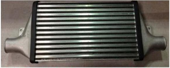
Apply the adhesive side of each of cushion strips along each side of the intercooler DIRECTLY ON TOP OF THE WELD BEADS and wrap around each corner to the top and bottom surfaces of each end tank. Please go back and pressure firmly down on the cushion strip to ensure adhesion
