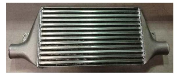
Clean the intercooler surfaces as detailed in the below picture, including the top and bottom sections
